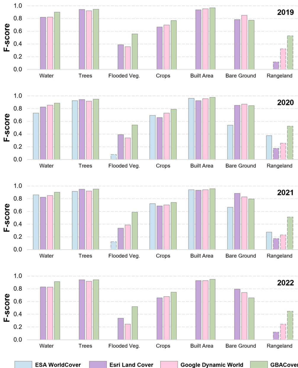
Fig. 5. Accuracy assessment results of the annual LULC products over different classes in 2019–2022. The annual LULC maps of ESA WorldCover in 2019 and 2022 are not available; thus, they are not involved in the comparisons. Meanwhile, the classification accuracy of wetlands in ESA WorldCover 2020 and 2021 is evaluated with the manual flooded vegetation labels and can only be relatively compared. Similar to Esri Land Cover products, the classes of grass and scrub are merged into rangeland for convenience of comparison among different products.
